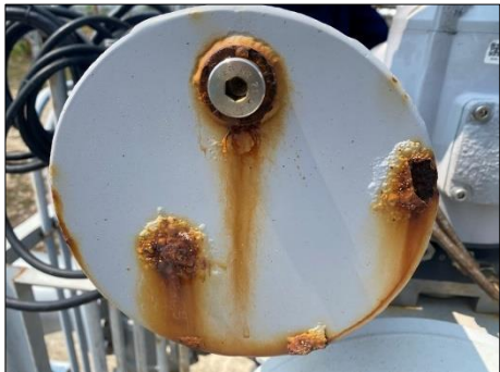
Fig 4. Was found Actuator reservoir corrosion.
