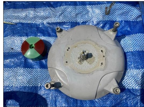
Fig 4. Check and cleaning switch indication cover.
