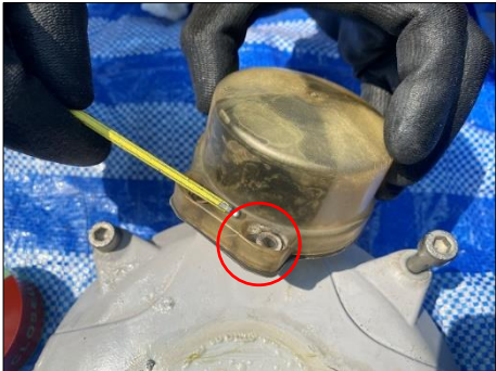
Fig 7. Switch indicator cover found broke.
