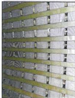
Figure 3: Stator Core
