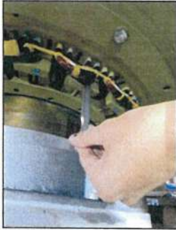
Figure 127: Air gap measurement (PMG Winding to PMG Pole)
