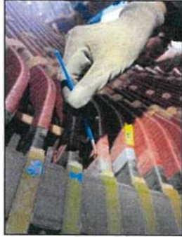
Figure 23: Stator Re-condition
