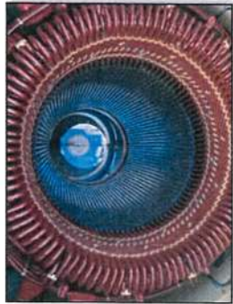
Figure 1: Stator Bore
