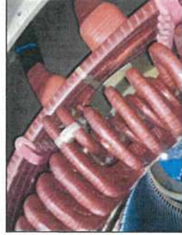
Figure 8: Insulation Series Connection
