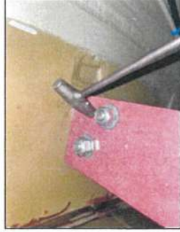
Figure 6: Taping Bolt End Winding Support
