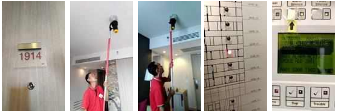
FL 19 ROOM 1914 TEST SMOKE DETECTOR 2 SET..NORMAL
