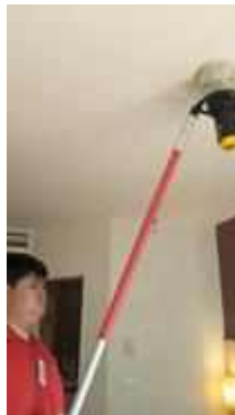
FL 17 ROOM 1726 TEST SMOKE DETECTOR 1 SET..NORMAL
