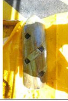
PIG good condition. No wax no sand.
