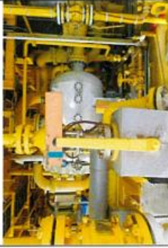
PIG indicator before pig arrived
