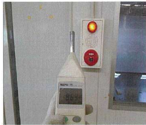
Combination Box (PLB) Testing and Decible
