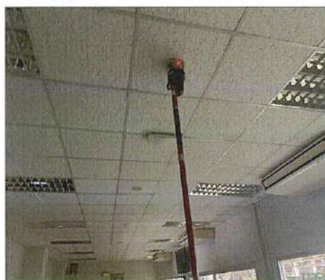
Heat Detector Testing
