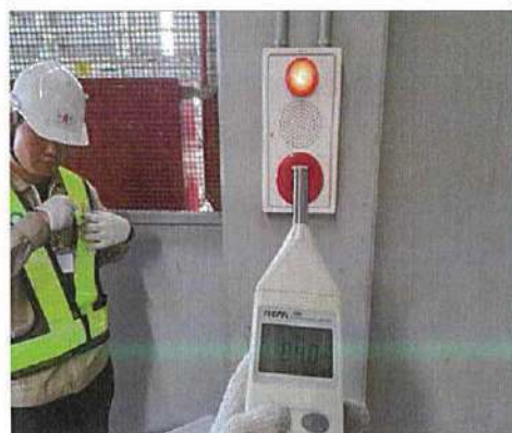
Combination Box (PLB) Testing and Decible
