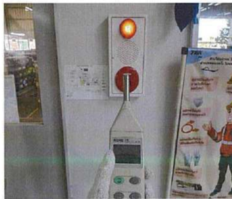
Combination Box (PLB) Testing and Decible
