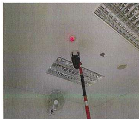
Heat Detector Testing
