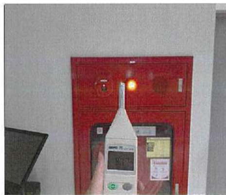
Combination Box (FHC) Testing and Decible
