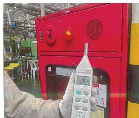
Combination Box (FHC) Testing and Decible
