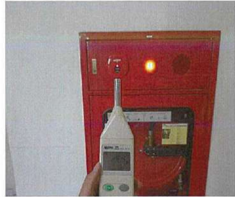
Combination Box (FHC) Testing and Decible
