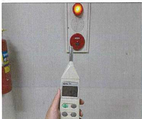
Combination Box (PLB) Testing and Decible
