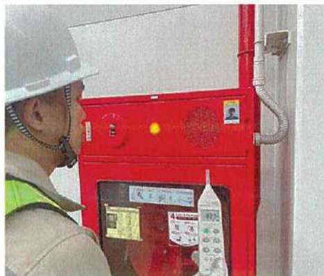
Combination Box (FHC) Testing and Decible
