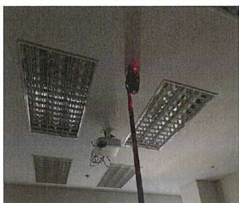
Heat Detector Testing
