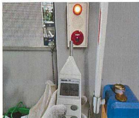
Combination Box (PLB) Testing and Decible
