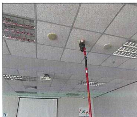
Heat Detector Testing
