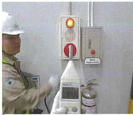
Combination Box (PLB) Testing and Decible
