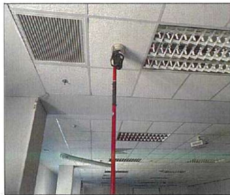
Smoke Detector Testing
