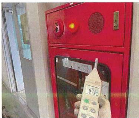
Combination Box (FHC) Testing and Decible
