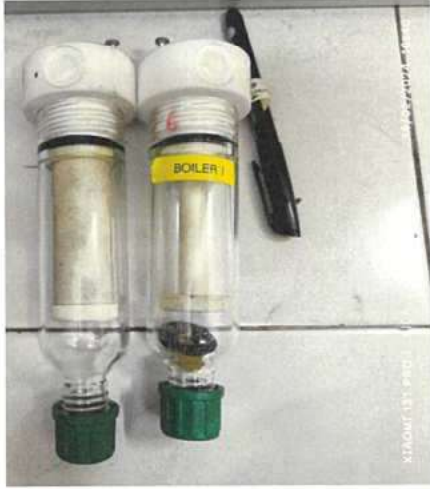
Model of moisture filter that replaced on boiler 1
