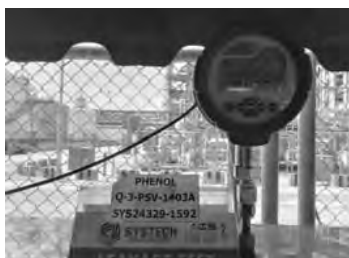
Initial Leakage Pressure Test
