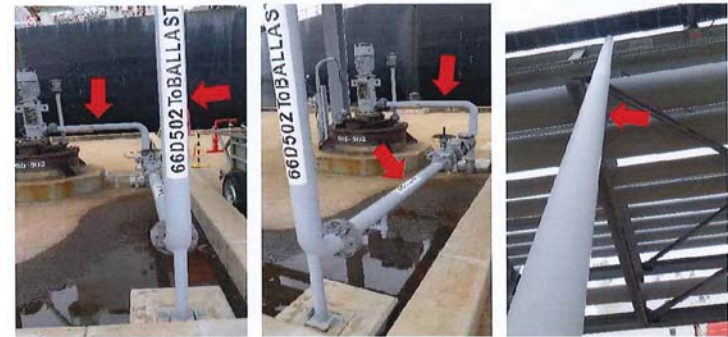
Photo13: 66D502 to ballast line still in good condition observed.
