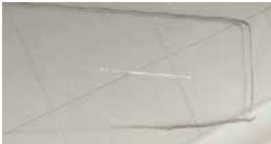
The drill rubbing the glass sample for appox 10,000 times.
