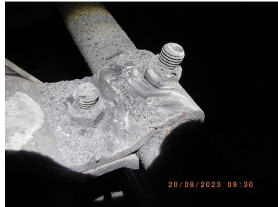
Picture 62 : Loose DE hammer bolt/nut
