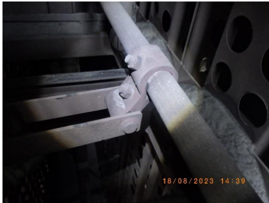
Picture 5 : Intact hammer clamp bolt/nut
