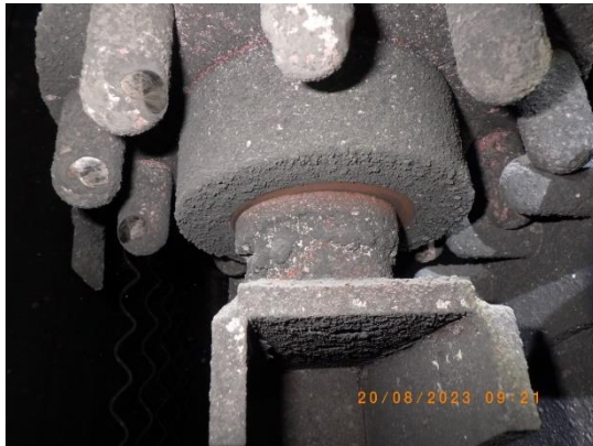
Picture 61 : DE horizontal and vertical pinwheels were in tolerable condition
