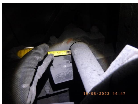
Picture 28 : Worn off CE bearing
