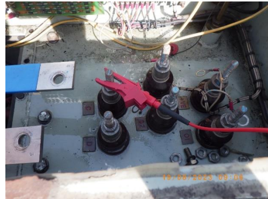
Picture 74 : HV – C phase insulation test
