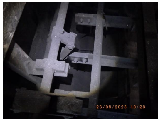
Picture 121 : Replaced CE anvil
