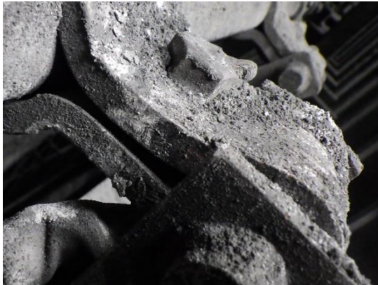
Picture 46 : Loose DE hammer clamp bolt/nut
