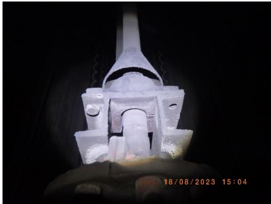
Picture 31 : DE vertical bearing still in tolerable condition
