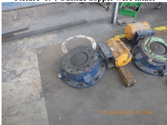
Picture 21 : Dome valve was found intact
