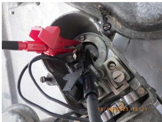
Picture 92 : Hopper heater resistance testing
