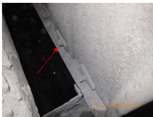
Picture 53 : Intact CE rapping bar bolt and nut
