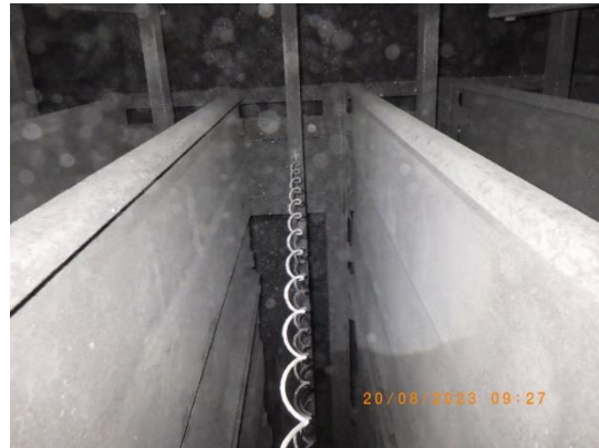
Picture 60 : All DEs were seen in tolerable tension and gap between CE-DE were normal
