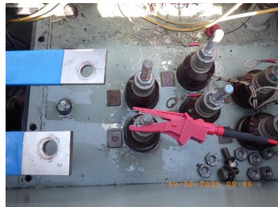
Picture 76 : HV – D phase insulation test
