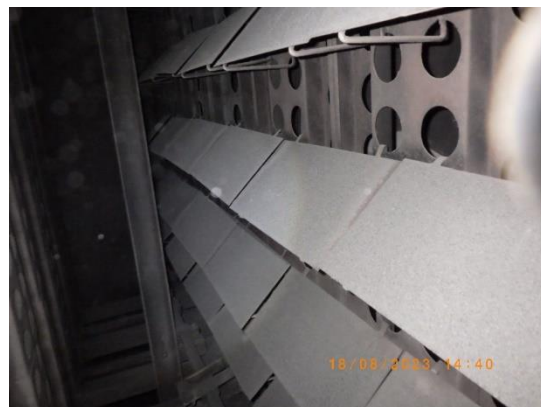
Picture 4 : Intact guide vanes on GD screen
