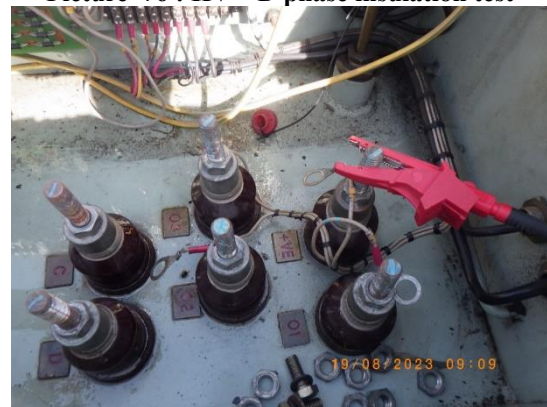
Picture 78 : HV – +VE (+) phase insulation test
