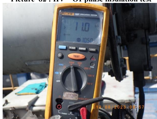
Picture 84 : HV - G phase insulation test
