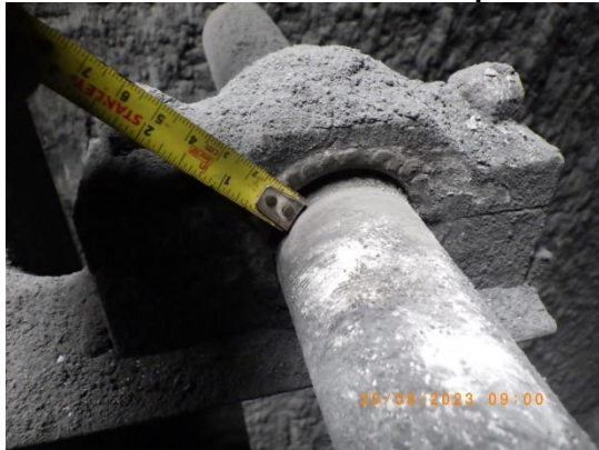
Picture 48 : Worn out horizontal DE bearing
