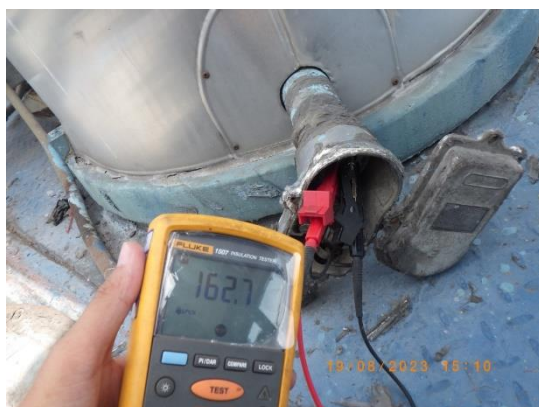
Picture 90 : Support insulator heater resistance testing
