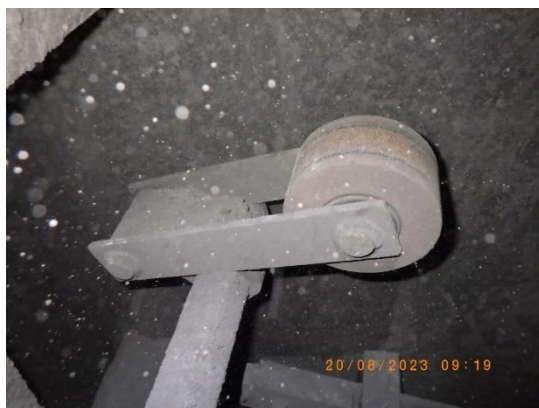
Picture 55 : CE hammer were intact
