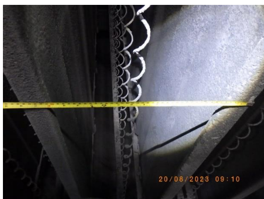
Picture 52 : Gap between CE-CE were normal
