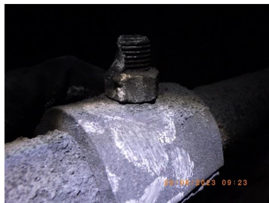
Picture 123 : Replaced DE hammer clamp bolt/nut
