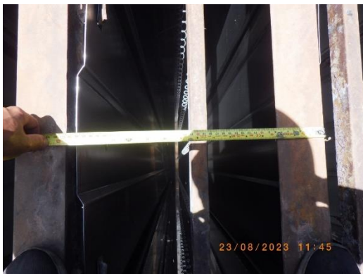
Picture 112 : Gap measurement between CE-CE at top portion
