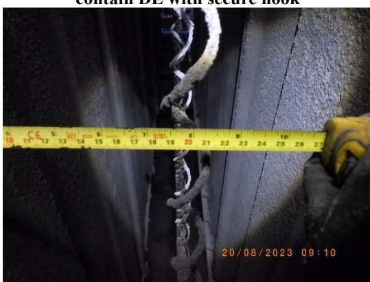
Picture 45 : Gap between CE-DE were in normal condition
