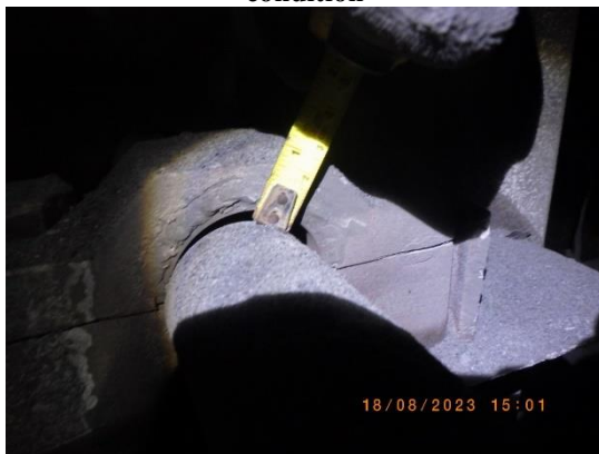
Picture 35 : Worn out horizontal DE bearing
