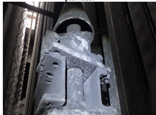
Picture 51 : DE vertical bearing was slightly worn off
