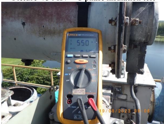
Picture 77 : HV – D phase insulation test
