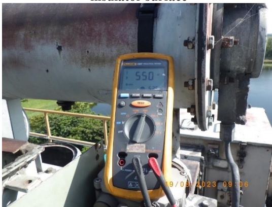
Picture 75 : HV – C phase insulation test
