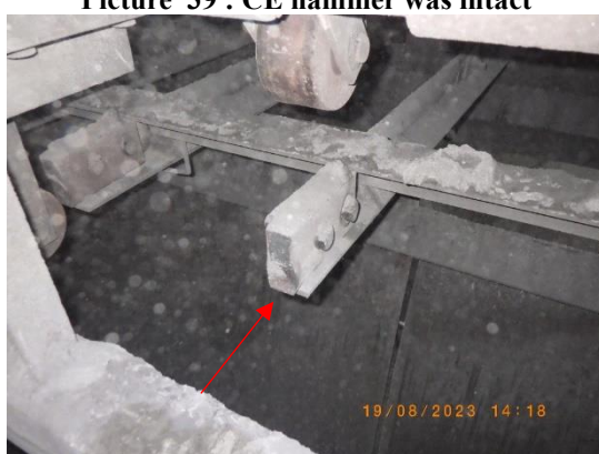
Picture 41 : Worn out CE anvil
