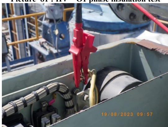
Picture 83 : HV - G phase insulation test
