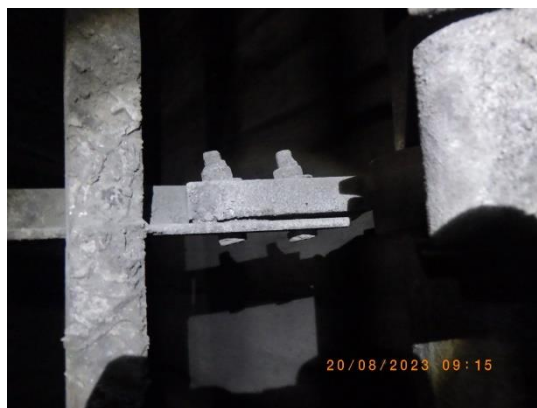
Picture 56 : Loose CE anvil bolt/nut
