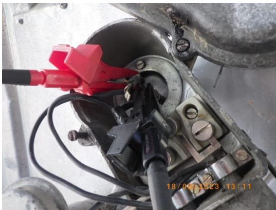
Picture 118 : Hopper heater resistance testing
