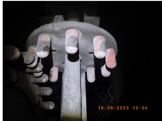
Picture 32 : Slightly worn off pinwheel
