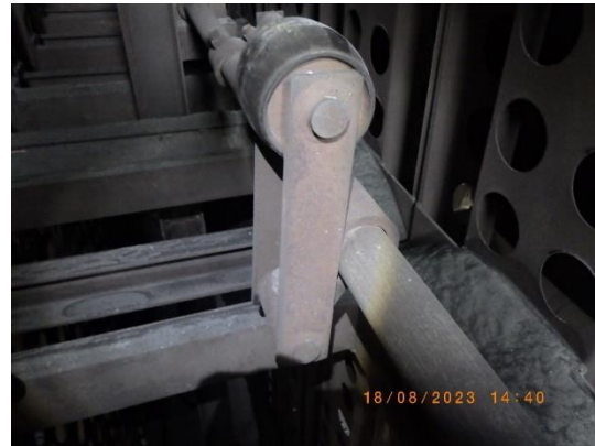
Picture 6 : Intact GD hammer
