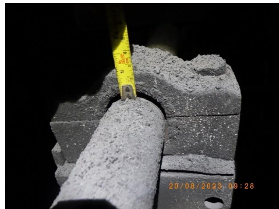
Picture 64 : Worn out horizontal DE bearing
