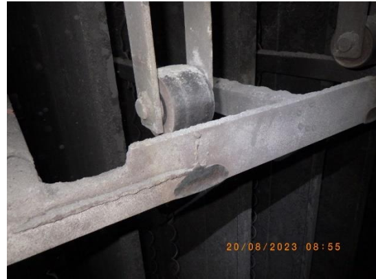
Picture 47 : Slightly worn off rapping anvil
