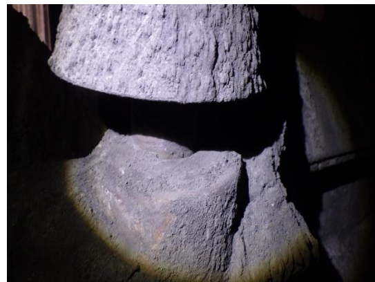
Picture 66 : DE vertical bearing slightly worn off
