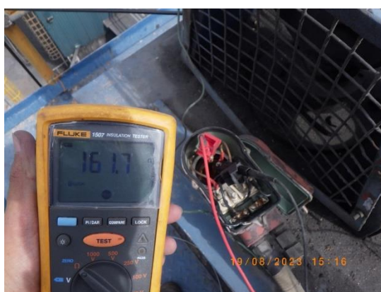
Picture 85 : Rapping insulator heater resistance testing
