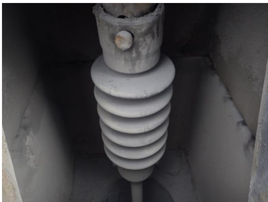
Picture 50 : DE rapping insulator in low position, worn out pinhole and dust accumulated on surface
