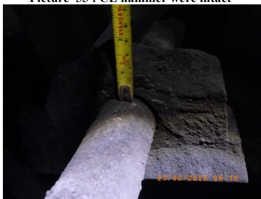
Picture 57 : Rapping bearing was still intact
