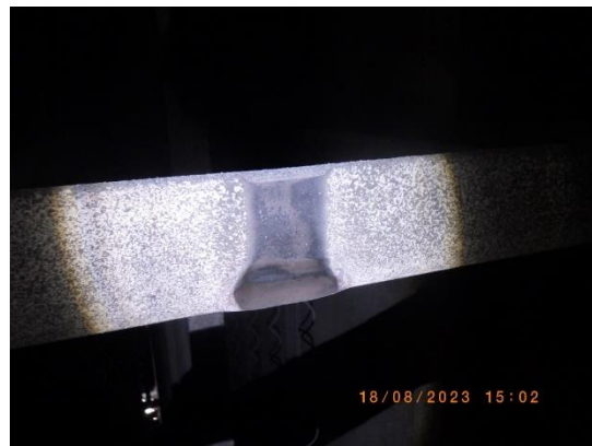
Picture 34 : Slightly worn off rapping anvil
