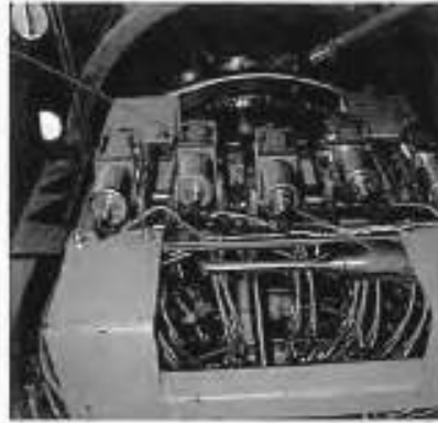
Figure 2: DLE Staging Valves
