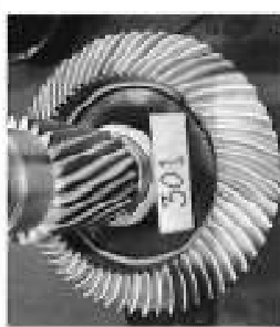
Inspect gear set by penetration test As found : Pinion scratched
