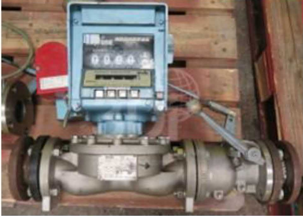
Figure 1. Flowmeter ready for calibration
