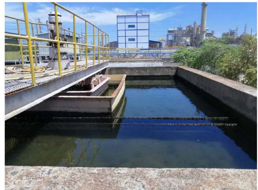
Clarify tank to precipitation method
