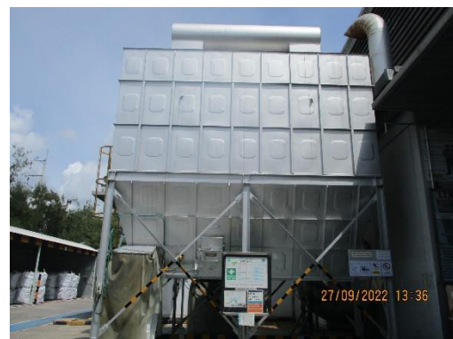
Dust Collector/Dross Recovery
