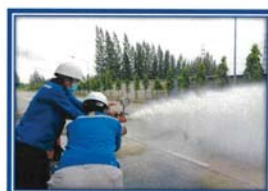
Picture shown : Testing by electric fire pump the flow of a fire hydrant with the valve fully open and record pressure.
