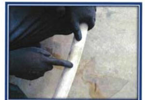
Picture shown : Maintain the pressure and inspect the fire water hose.
