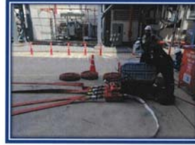
Picture shown : Prepare tools and fire hose for hydrostatic test fire hose.
