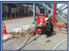
Picture shown : Hydrostatic test rack hose polyester single jacket and maintain the pressure 250 PSI.
