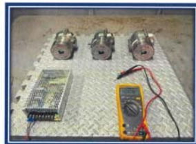
Picture shown : Inspection flame detector and remove out the device to testing at workshop.
