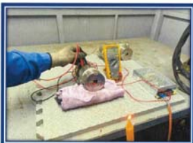
Picture shown : Testing the flame detector at workshop and device working properly.
