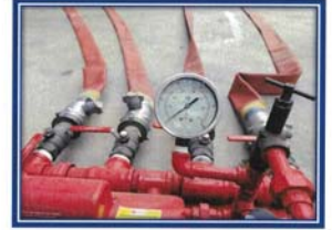
Picture shown : Prepare tools and fire hose for hydrostatic test fire hose.
