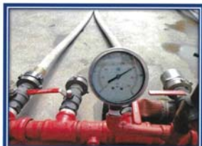
Picture shown : Hydrostatic test rack hose polyester single jacket and maintain the pressure 250 PSI.
