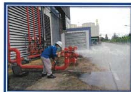
Picture shown : Testing by engine fire pump the flow of a fire hydrant with the valve fully open and record pressure.
