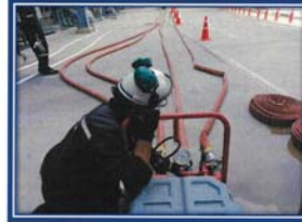
Picture shown : Hydrostatic test fire water hose Rubber Lining fire hose and maintain the pressure at 250 PSI.
