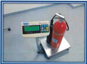
Picture shown : Inspection and weight check CO2 portable fire extinguisher.
