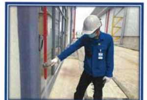
Picture shown : Function test automatic sprinkler system by drain test at Office Admin Building.
