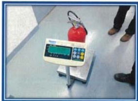
Picture shown : Inspection and weight check CO2 portable fire extinguisher.
