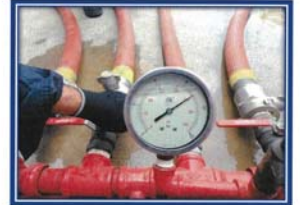
Picture shown : Hydrostatic test fire water hose Rubber Lining fire hose and maintain the pressure at 250 PSI.
