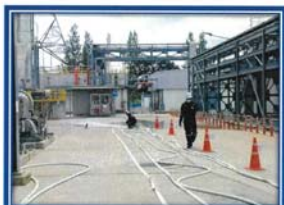
Picture shown : Picture shown : Hydrostatic test fire water hose.
