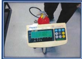
Picture shown : Inspection and weight check CO2 portable fire extinguisher.
