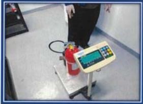
Picture shown : Inspection and weight check CO2 portable fire extinguisher.
