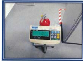
Picture shown : Inspection and weight check CO2 portable fire extinguisher.
