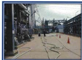
Picture shown : Hydrostatic test fire water hose type Rack Hose polyester single jacket.
