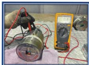
Picture shown : Testing the flame detector at workshop and device working properly.
