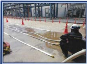
Picture shown : Hydrostatic test fire water hose type Rack Hose polyester single jacket.
