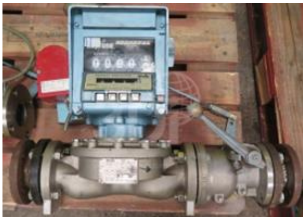
Figure 1. Flowmeter ready for calibration
