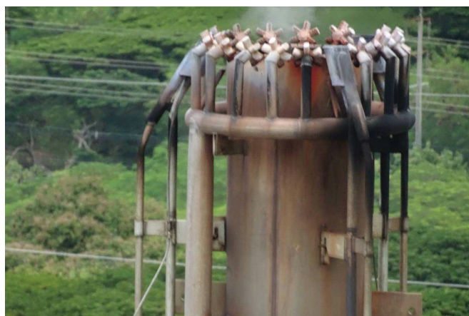
Figure 13: Flare Burner of elevated flare.
