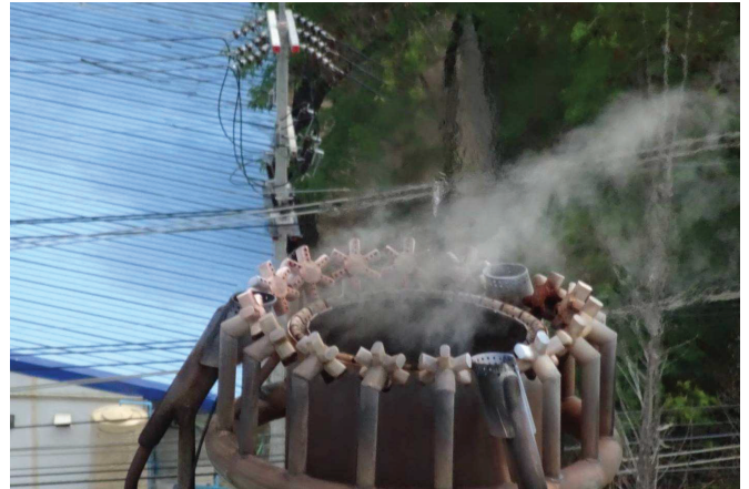
Figure 15: Flare Burner of elevated flare.
