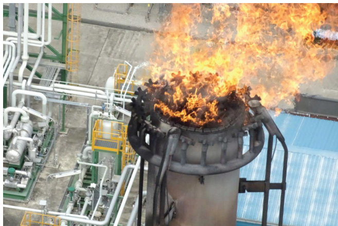
Figure 31: Flare Burner of elevated flare.
