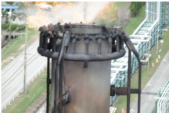
Figure 30: Flare Burner of elevated flare.
