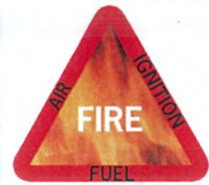
THE FIRE TRIANGLE, ALL THREE ELEMENTS: FUEL/AIR/IGNITION MUST BE PRESENT FOR IGNITION TO OCCUR
