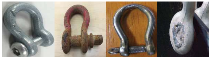
Gap/Wounds/Crack Severe Rust Abrasion thermal strain(Welding)
