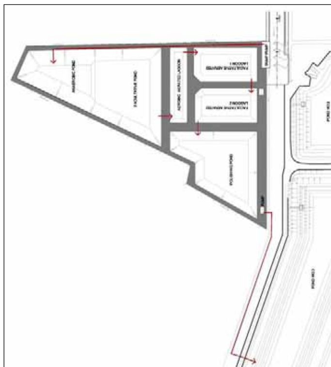
LAY OUT PLAN OF WASTEWATER TREATMENT PLANT (capacity 2,800 m. 3 /d)
