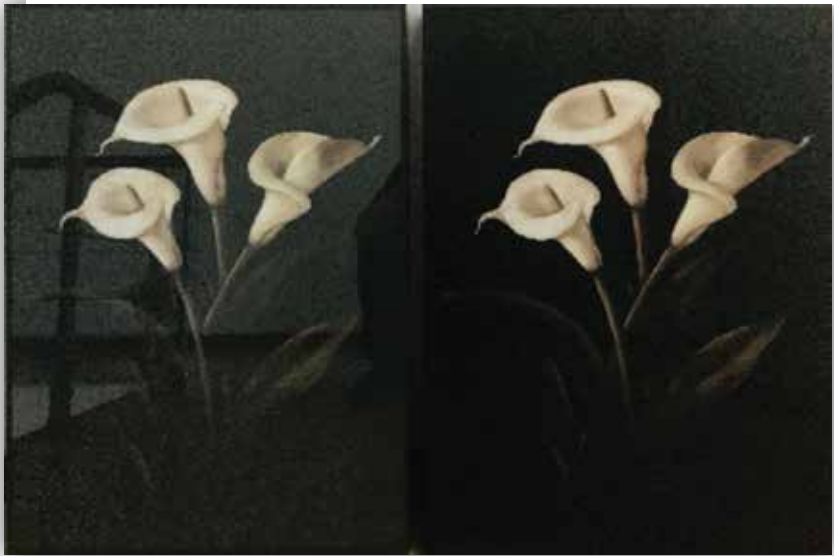
Image observed from a Glass without Anti-Reflective coating
