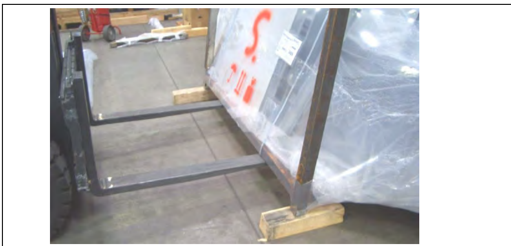
Fig.: 21 - Tilting of storage rack
