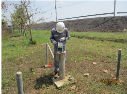
GWR1 Up Gradient Monitoring Well
