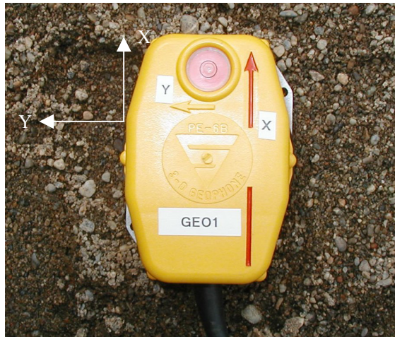
Figure 2 Geophone, showing orthogonal directions of velocity measurement
