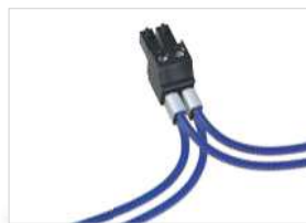
Fig.: 2-pole plug contact with cable connection (cable type: 2 x 0,75 mm 2 ) via twin core end sheathes
